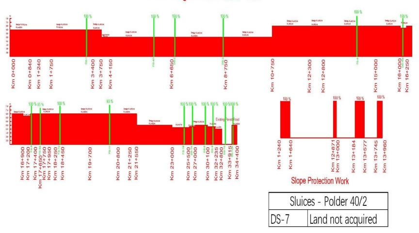
Figure 3-25: Line Diagram of Polder-40/2
